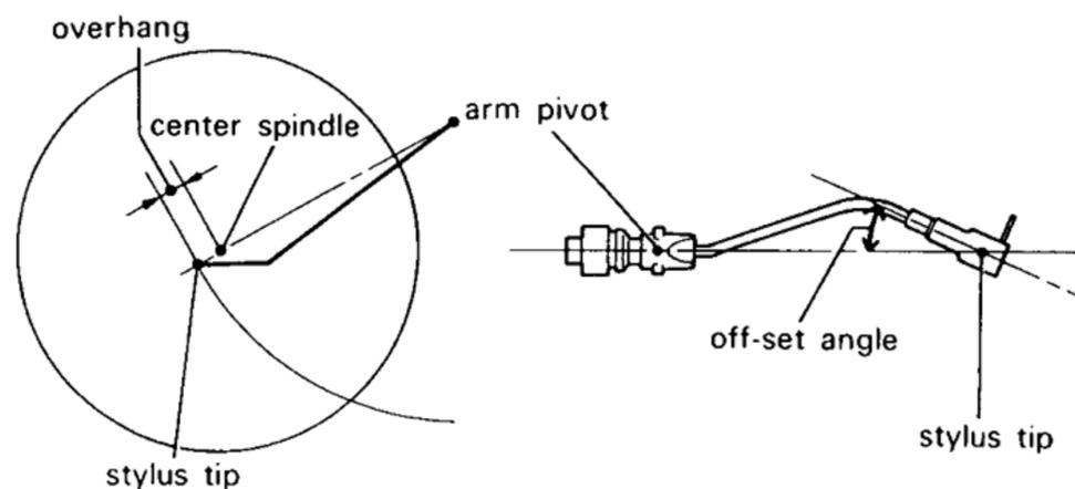
Tracking error is minimized by the selection of an optimum "off-set" angle and "overhang" distance. Overhang is the distance between the stylus tip and the center spindle. This overhang adjustment is made at the time of installing a particular cartridge, while the off-set angle is fixed by the manufacturer of the tonearm.
